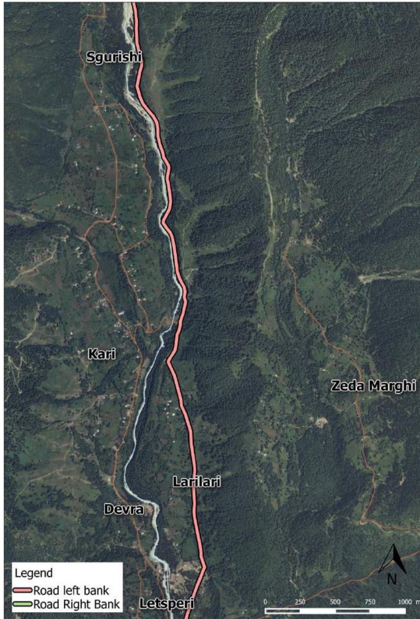
Figure 29 - Proposed alignment of access road to the dam to be upgraded - Letsperi to Tita
