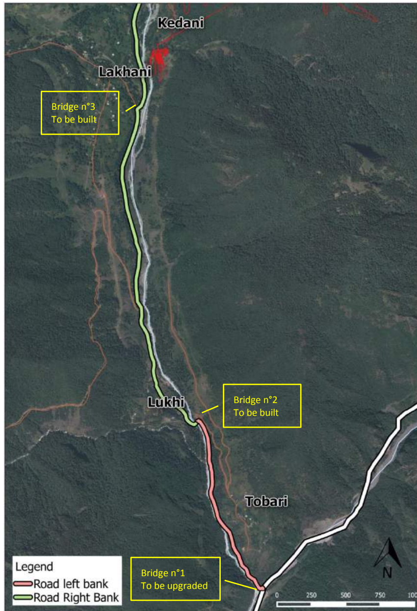
Figure 29 - Proposed alignment of access road to the dam to be upgraded - Enguri to Letsperi
